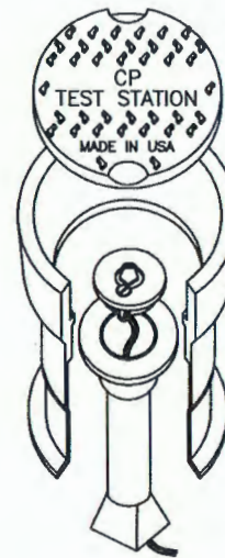
SNAKEPIT & VALVE BOX TOP ASSEMBLY
